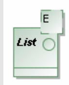
Figure 37 -- UML Interface representing “java.util.List” with template parameter
